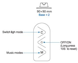
If you don't have Wi-Fi at home or cannot pair it for some reason but still want to use this light, simply wait for 3 minutes for the light to stop blinking, then manually press C button on Wi-Fi controller to change colour and modes
