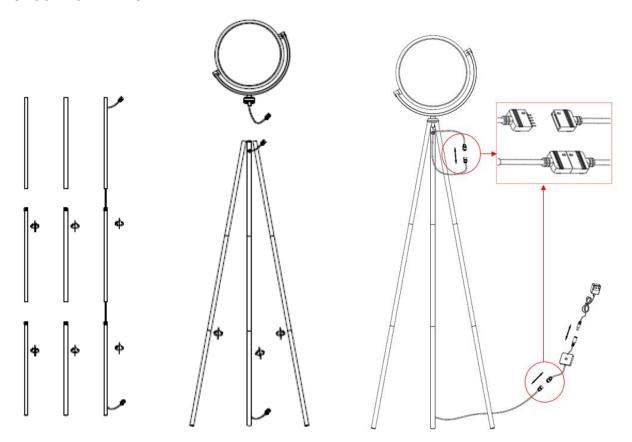
When connecting the Floor lamp to the Wi-Fi controller, make sure the two arrows are aligned with each other.
