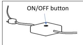
If you having difficulty connect this lamp to the Genio APP, wait for 3 minutes and lamp stopped working, you can control this lamp manually using the button on Wi-Fi controller.
