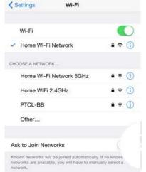
To verify your mobile phone is connected a 2.4Ghz Wi-Fi network, navigate to the **Setting** menu and click on **Wi-Fi.** In this menu you will see all detectable networks in your area. Locate the SSID for your network, select a Wi-Fi SSID that doesn't end with 5GHz.
