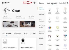
3. Follow the APP's instructions carefully to complete the network pairing process. Please make sure you are using the 2.4Ghz Wi-Fi name and password.
