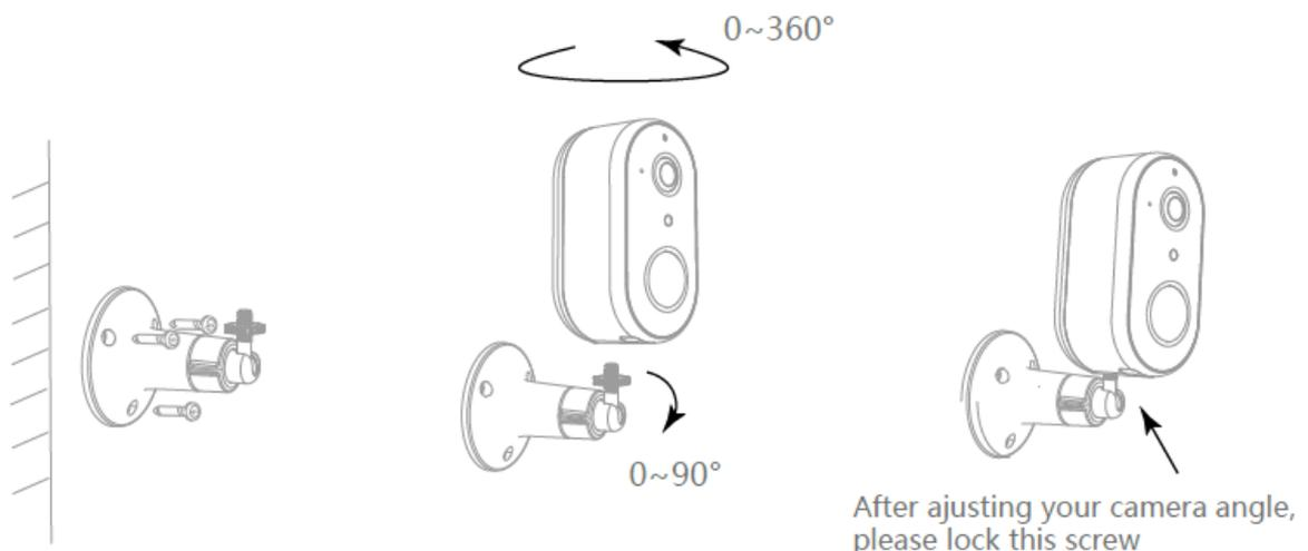
1. Fix the bracket on the wall
