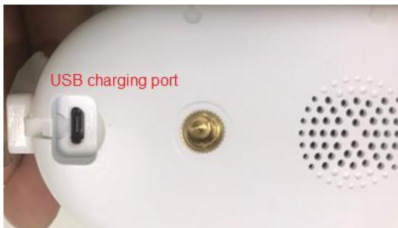
**Note:** battery can be recharged with the supplied USB cable and standard 5V 1A mobile phone USB adaptor (not included)
