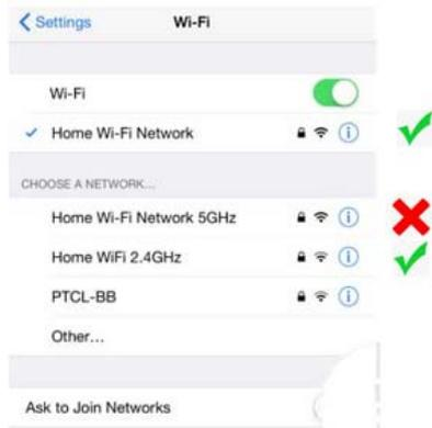
Once you have confirmed that you have selected the 2.4GHz network, check that you have a strong WI-FI signal (at least two bars) in the location where the smart device is to be installed.
